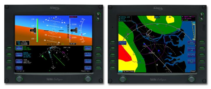
The FlightMax Entegra primary flight display (PFD) and multi-function display (MFD) are designed to provide pilots with all the information needed to manage the aircraft and safely determine routes, speeds, as well as proximity to adverse weather conditions, terrain, obstacles, and other aircraft.
